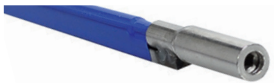
Boston double action truss rod 42247 TRD-590-4 6x9mm bar model, 4mm allen nut, 590mm length, for bass guitar
