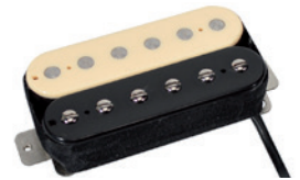
Boston Power Rock humbucker pickup, Alnico 5 bar, 4 conductors, waxed formvar wire, 9.6K neck, zebra
