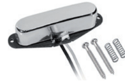
Boston Vintage single coil pickup, Alnico 5 rods, black fibre bobbin, waxed formvar wire, 7.5K, neck
