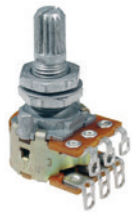
ALPS 2x250K blender potentiometer 14110 PM-250-Z 10mm. bushing, M7x0,75 thread, blends 2 sources, made in Japan
