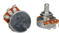
Alpha 250K linear potentiometer 31830 ALP250-B36 solid shaft, short bushing .250", 3/8" diameter, for pickguard mount
