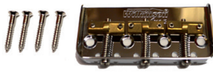
Wilkinson bridge-tailpiece Teaser short version, pitch 10,8mm, staggered brass saddles
